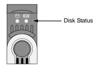
Figure 9. VTrak M500f/i/p disk carrier LEDs
